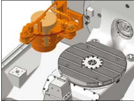
Head separated type Renishaw NC4S · Blum MICRO SINGLE NT
