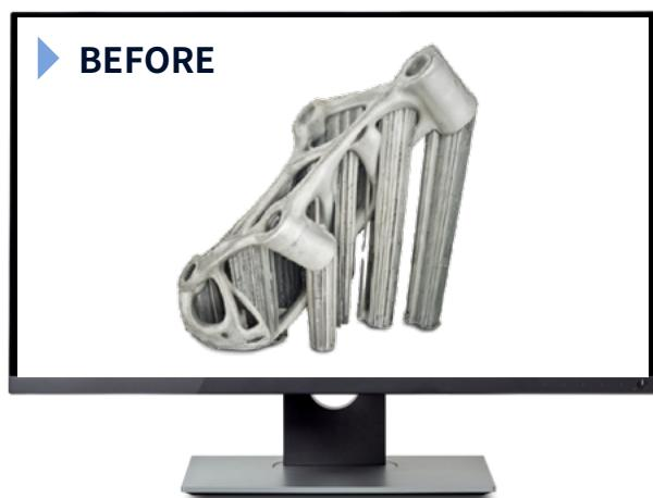
Manufacturing of a bracket on a DLX 150; Material: SS316L, Part Volume: 8.5 cm<sup>3</sup>
